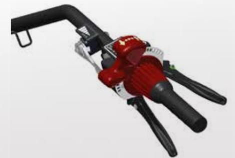
For both forwarding controls, a notch sector allows the operator to easily and repeatedly fix the position of the lever or of the knob. A central area without notches lets the lever or the knob to be positioned as desired, so that the machine can operate at a very slow speed.
